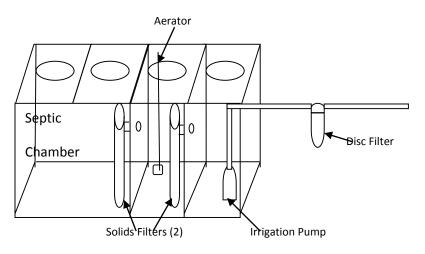
In order to flush/purge the lines it is necessary to open the purge valves or flush taps at the end of each disposal line and to activate the pump in the pump chamber. The reason for doing this is to prevent the lines becoming blocked with an excess build up of biomass. Sometimes it is better to flush the lines one at a time, in order to keep the pressure up and get the biomass out of the lines. Once the line runs clear water then it can be closed and you can move onto the next one.
