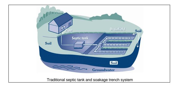
Traditional septic tank and soakage trench systems worked well for large lots (1/4 acre or more), but had limitations in clay soils (poor soakage conditions) or gravelly soils (too rapid soakage resulting in pollution of wells). For small lot subdivisions, septic tank effluent resulted in groundwater contamination in some locations. Un-maintained septic tanks exacerbated these problems.
